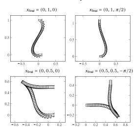
solution trajectories with different final states; the outline of the car shows the position  $(p_1(kh); p_2(kh))$ , orientation  $\theta(kh)$ , and the steering angle  $\phi(kh)$  at time kh
