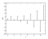
although the input is bounded and quickly decays to zero, the system itself is unstable and an unbounded output results
